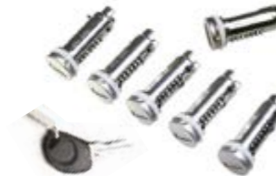
OYS-910 IVECO III - IV KEY PROFILE: GT10 OEM: 299651P
