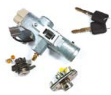
OYS-NS013 TIIDA (05-11) AT LHD / VERSA / LATI0 / DG TRAZO (05/11) KEY PROFILE: NSN14 OEM: 99810-ED800-B116
